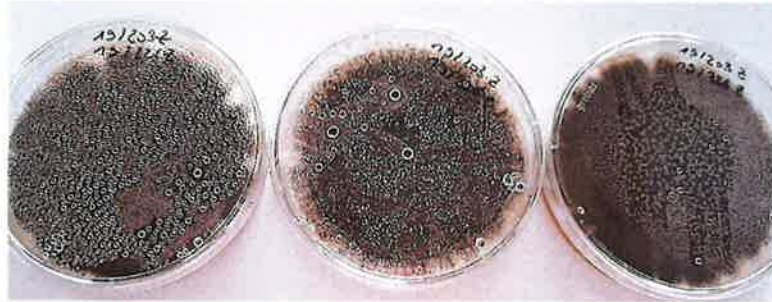
Controls are covered by mould
