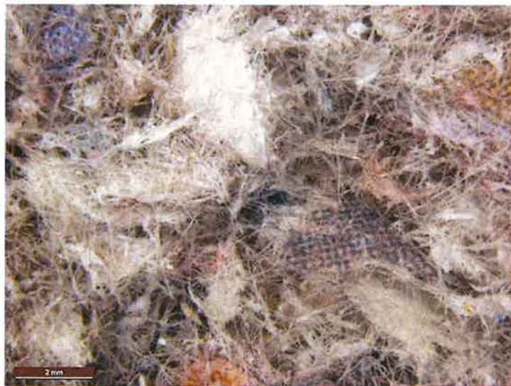
Microscopic aspect of the insulation product (magnification x 7.8)
